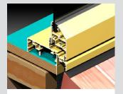
The frame is 102mm thick with 40mm thick sashes that are strong enough for exposed locations. We have several sash options to choose from.
